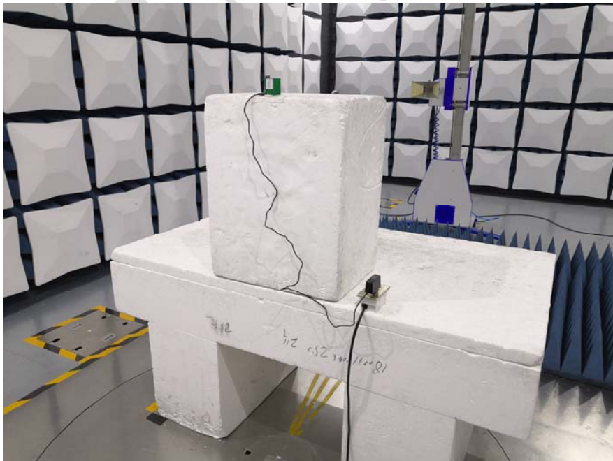
Radiated Spurious Emissions View (Above 1 GHz)
